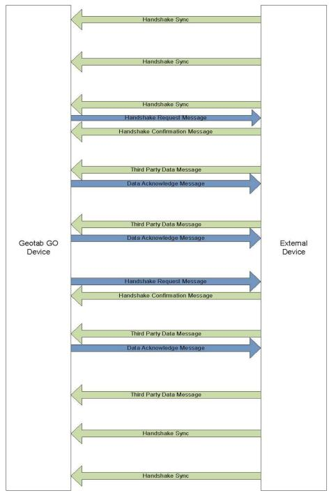
Fig 1: Example of External Device Message Flow
